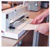
Now put the project to be creased into the creasing/cutting slot. Push the handle partly down to hold the project in position. Ensure it's square and in position. Now press harder to make the crease.
