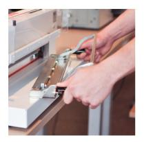
Ensure the guillotine and paper clamp handles are in the open position, now lift the safety guard up, fit the creasing tool in the cutting slot.
