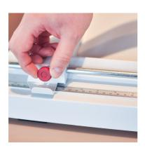
Use the back adjustable guide to set the creasing position.
