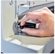
Regulate the device with the thumbscrews so it is square and parallel against the paper clamp. Make a test with a plain piece of paper.
